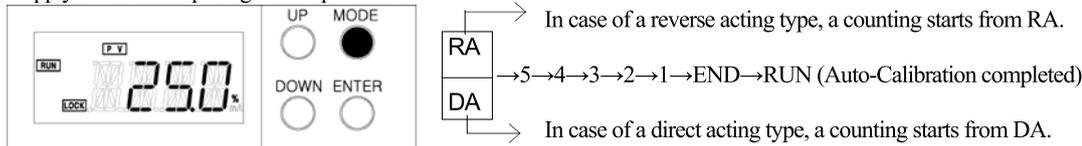
**▲ Time required for this Quick Auto-Calibration process may be different according to the control valves, but it generally takes about 2~3 minutes. In case of a large-sized actuator, more time is required to wait.**
